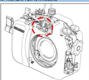
Install the camera body into the housing first and mount the optical fiber cables to the housing in the case of using strokes
