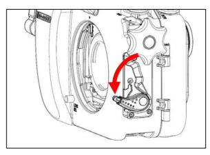
2. Turn the port locking lever of the housing to the release position as shown.
