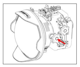
5. Engage the focus gear on the lens by pushing the knob inwards, then turn the knob both ways to check if the lens is functioning
