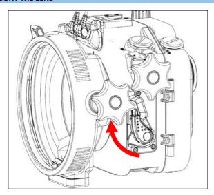
1. Lock the adaptor into place by turning the port locking lever of the housing to the inward position. To ensure that the adaptor is securely mounted, confirm that the green line on the safety button of the port locking lever is visible.
