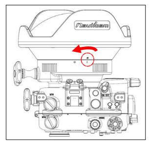
Align the "I" mark on the adaptor with the WHITE dot on the port. Gently push the port towards the adaptor until it cannot go in any further.
