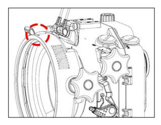
3. Align the port mounting indicates of the N85 to N120 50mm port adaptor II and the housing.
